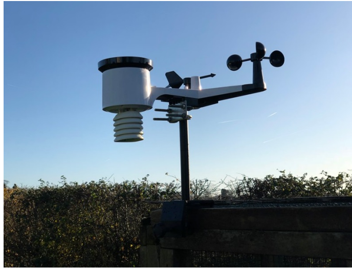
Figure 3.14: B-Fluid On-site Weather Station
